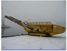
Used at the docks, the hopper buffers and takes care of a even load flow into the vessel.
