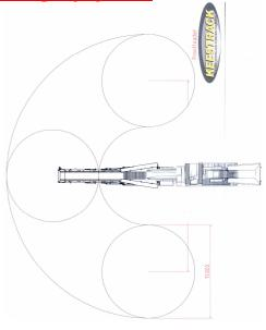
Rotating storage transporter. Can turn around it own axis on tracks while running and can stock Ca. 3.500 ton in 270 degrees.
